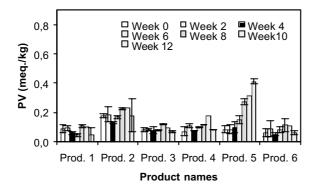
enzymatic interesterification (Prod. 3 storage. Based on PV, adding fish oil has major effects on product oxidation stability during storage. PV for the butter spread containing fish oil without adding antioxidant (Prod. 5) after 8 weeks storage was twice as high compared with the other products.
