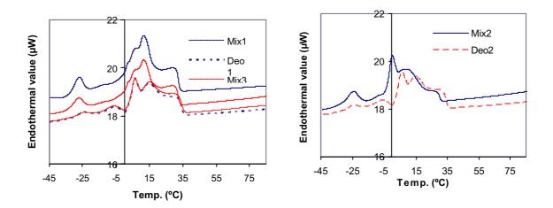
From SFC results, it can be seen that the changes of SFC at 5 °C after interesterification were increased and more pronounced for higher content of BF in the blends. The melting behaviours of different blends (**Figure above**) and interesterified products (**Table below**) were affected by amount of BF in the blends (Mix1 and Mix3 were close to each other).
