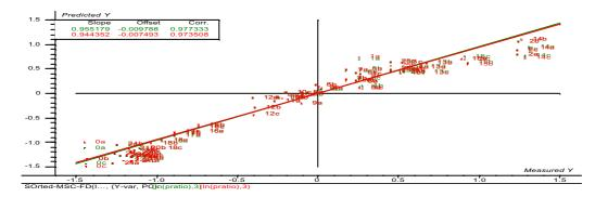
An improved validation model (**Figure above**) was obtained with coefficient of 0.938 at spectra range of 4513-12019 cm<sup>-1</sup>. By narrowing down the spectra range of 4513-5269 cm<sup>-1</sup>, coefficients were 0.977 and 0.974 for calibration and validation models, respectively. The standard error for the validation model was 0.186.
