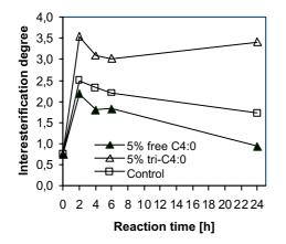
Short-chain fatty acids, such as butyric acid, which butterfat contains (10.8%), are more hydrophilic and they lower the pH of the microaqueous layer surrounding the enzyme, which may lead to enzyme deactivation in the free forms (Left Figure). Therefore, water content should be minimised to lower the hydrolysis reaction in the system. The effect was observed to be minimised in longterm operations where water content is reduced and stabilised.
